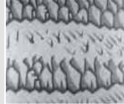
Magnetic domains on a silicon-iron electrical sheet Kerr microscopy EC Epiplan-NEOFLUAR 20x/0.50
