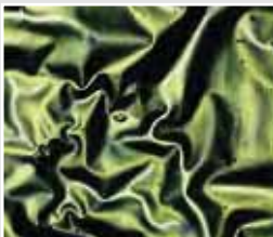
Layer of gold detaching from a silicon wafer Brightfield ACHROPLAN 10x/0.25
