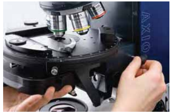
The stage carrier can be removed or its height adjusted by hand.
