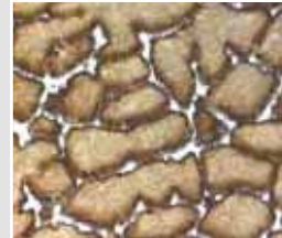
Maraging steel recast structure, nital etch with white, unetched areas Differential Interference Contrast EC Epiplan-NEOFLUAR, 50x/0.80
